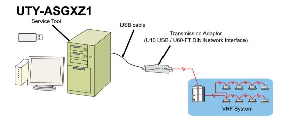
This transmission adaptor U10 USB / U60-FT DIN Network Interface is connected using the USB port of a personal computer.
