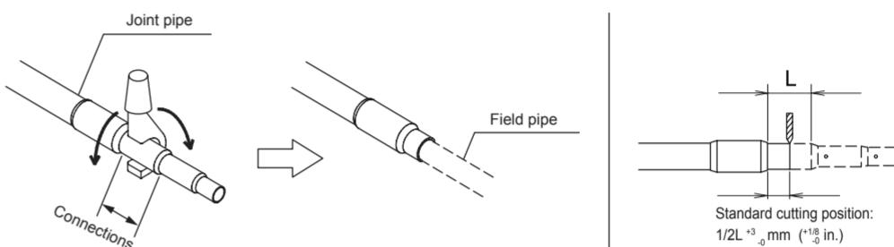
NOTE: Insert the field pipe firmly until it touches the joint pipe (Branch kit).
