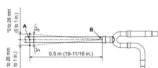
\*: Allowed value based on "A" (center of field pipe) at 0.5 m (19-11/16 in.) from "B" (junction of the branch kit).
