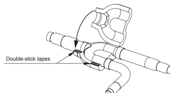
2) Be sure to install the tape (Accessory) in each heat insulation to the 2 positions as shown in the following figure.
