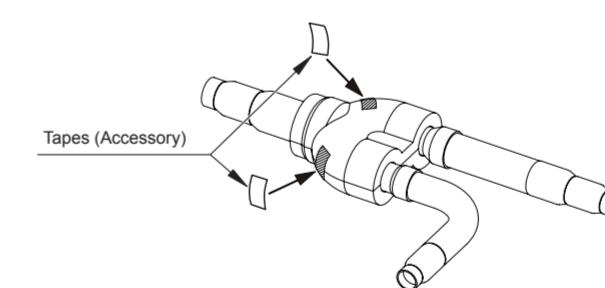
3) Use tape (Field supply) to seal the seam so that there will be gap at the junction between the aforementioned heat insulation and the heat insulation on the local piping.
