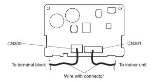
• Connection depends on the PCB type of the indoor unit. Refer to the installation manual of the indoor unit for details on how to connect to the indoor unit PCB.
