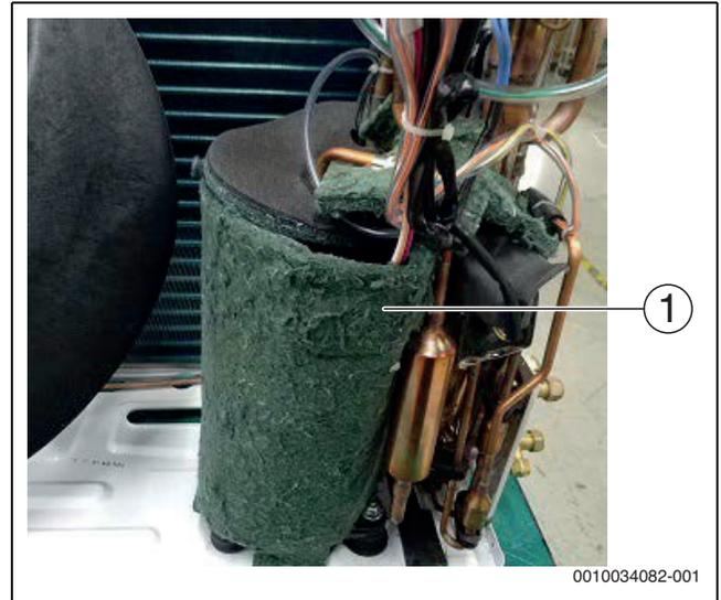
Fig. 148 Removing compressor cover 1
