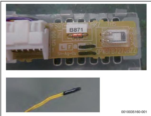
Fig. 171 Room temperature thermistor
