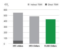
TEWI over a 15-year life cycle of a 100 kW refrigeration chiller. Calculation of electricity consumption according to Ecodesign. Annual leakage rate of 5 %. Emission factor 0.15 kg CO<sub>3</sub>/kWh.
