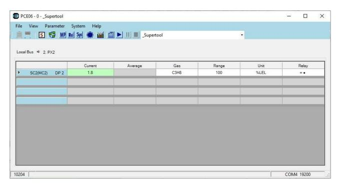
Exit the Special mode by pressing the Substant button or un-checking "Special mode" under "System" menu.
