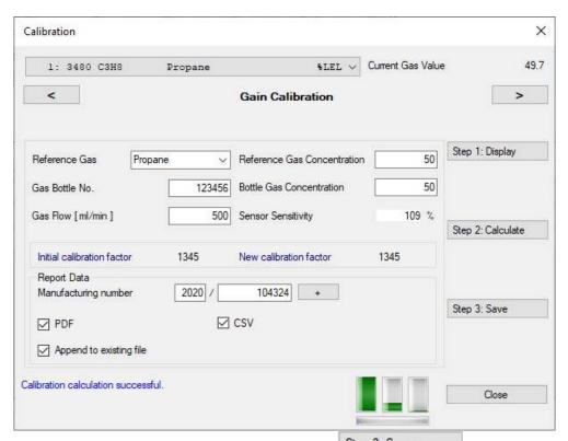
Continue with data saving by pressing the button Step 3: Save and after the data has been saved, the message indicating the folder with the saved file is displayed. See in the example, the message: "The file C: \ Calibration \ PX2-CH3-report.csv has been saved successfully".
