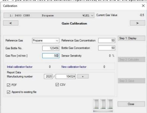
Make sure that the adapter is screwed onto the sensor head and the gas cylinder connected with the appropriate tube, then open the tap of the flow meter by delivering gas to the sensor. Press the button Step 1: Display
