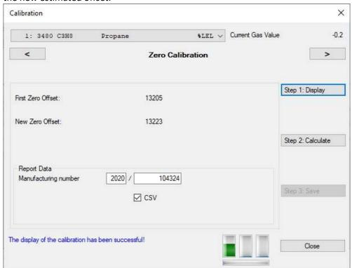
If the operation is successful, the following message is shown in blue on the screen: "The display of the calibration has been successful".
