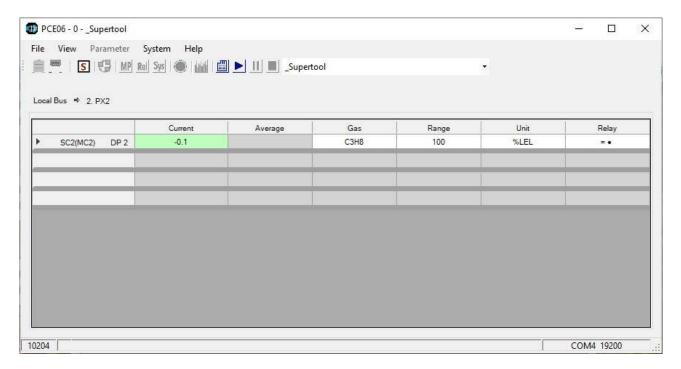
At this moment the sensor is in the normal operating state. To proceed with the calibration, one must enter the "special" state, by pressing the button , or by clicking "Special mode" in the System menu.
