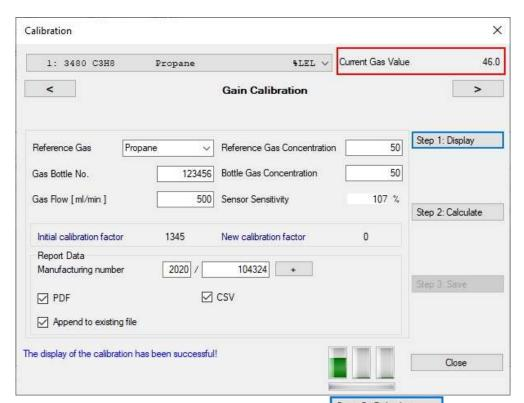
When the value begins to stabilize, press the button Step 2: Calculate and wait for feedback. If the reading concentration continues to change, the message will be "Sensor stabilization time running .." notifying that the calculation is still in progress:
