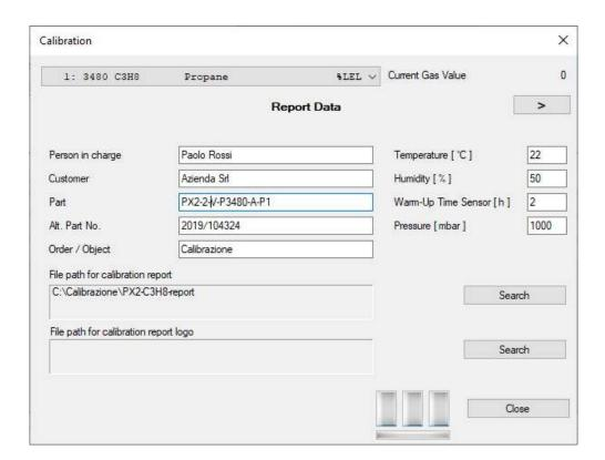
Once the data has been filled in, press the arrow button \_\_\_\_\_, to the right of the "Report Data" label and the zero calibration dialog box opens.
