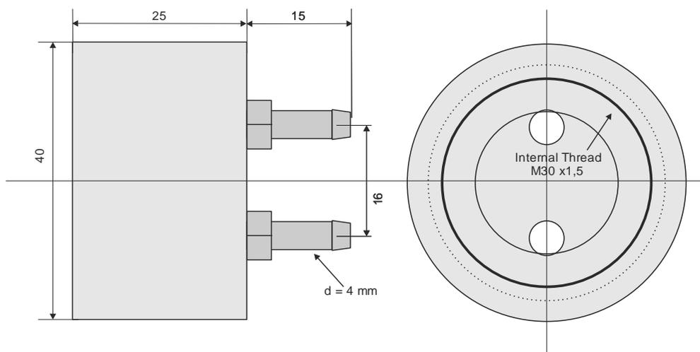
Fig.13.1: Calibration Adapter
