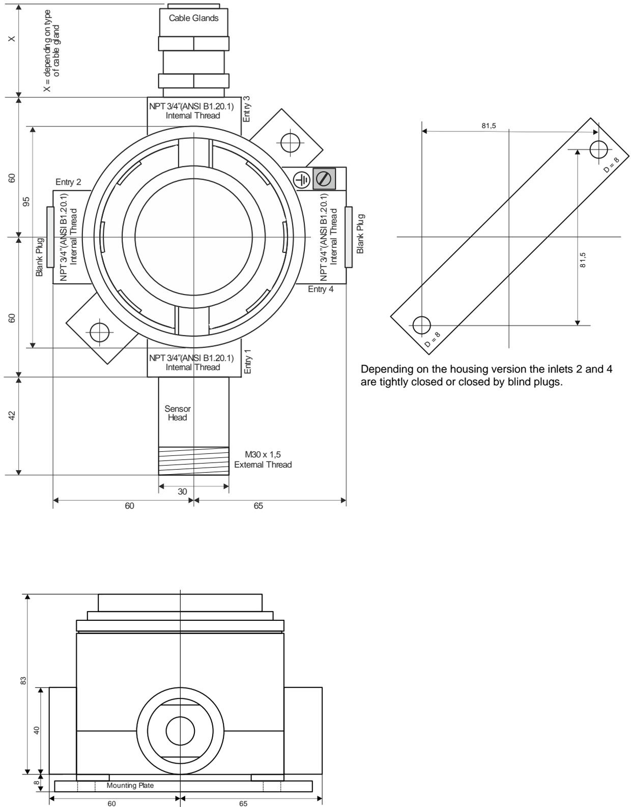
Fig.3.1: Dimensions and Mounting
