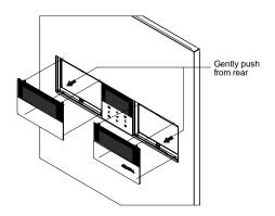
2 Remove the 4 screws and take out the holder with Remote Controller  $\widehat{1}$ .
