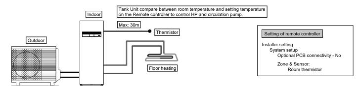
Connect floor heating or radiator directly to Tank Unit.
