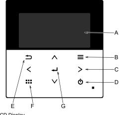
Name **Function** A: Main screen Display information Open/Close main menu B: Menu Select or change item C: Triangle (Move) Start/Stop operation D: Operate E: Back Back to previous item Open/Close Quick menu F: Quick Menu G: OK Confirm
