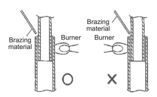
The pre-heating is to heat the base material until the melting temperature, and requires certain training to distinguish the color of the heated base material in order not to melt the material. The color and temperature of copper tube
