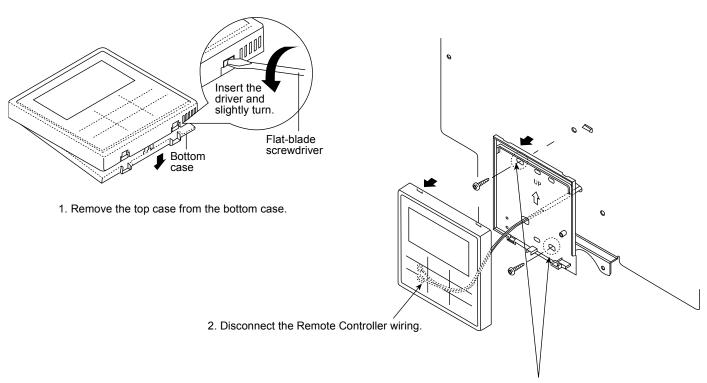
3. Remove 2 screws then take out the bottom case.
