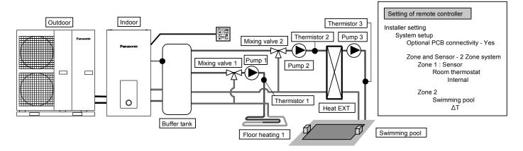
Connect floor heating and swimming pool to 2 circuits through buffer tank as shown in figure.
