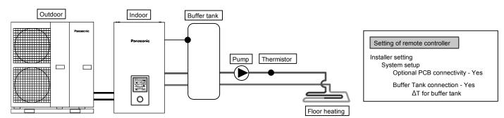
This is an application that connects the buffer tank to the indoor unit. Buffer tank's temperature is detected by buffer tank thermistor (specified by Panasonic). This system requires optional PCB (CZ-NS4P).
