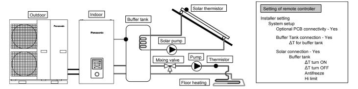
This is an application that connects the buffer tank to the indoor unit before connecting to the solar water heater to heat up the tank.
