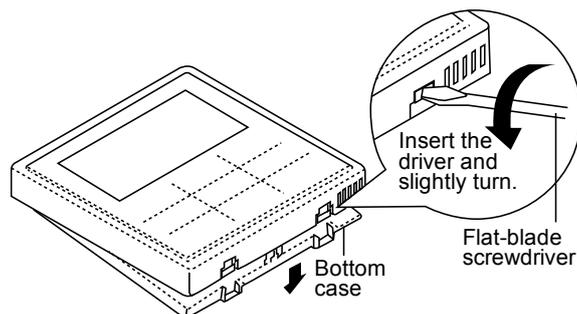
2. Remove the wiring between Remote controller and Indoor Unit terminal. Remove the bottom case from the Control board cover by loosening the screws. (3 pieces)
