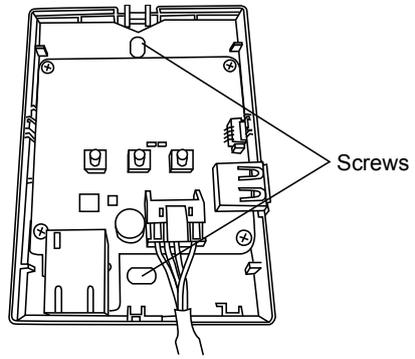
4. **Pull the CN-CNT cable through the hole in the bottom of the adaptor and re-attach the front cover to the back cover.**
