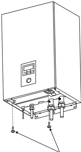
1. Remove the 2 mounting screws which located at bottom of the front plate.
