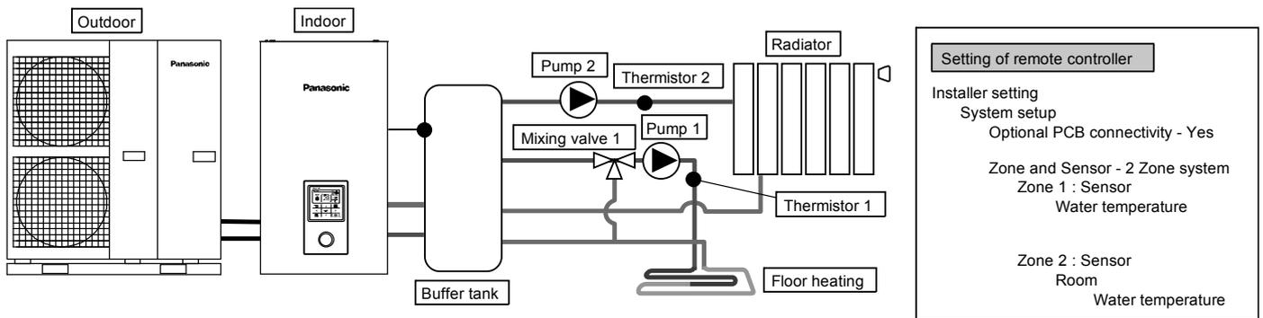
Connect floor heating or radiator to 2 circuits through buffer tank as shown in figure.
