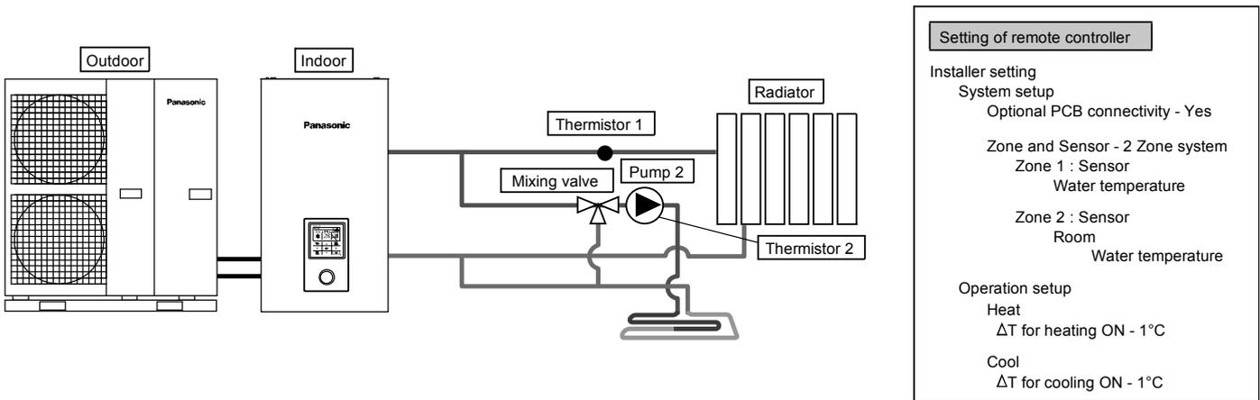
This is an example of simple 2 zone control without using buffer tank.
