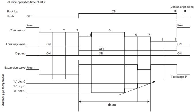
\* Backup heater must Turn OFF if the water pump turn OFF.
