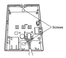
4. Pull the CN-CNT cable through the hole in the bottom of the adaptor and re-attach the front cover to the back cover.
