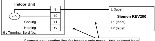
Connect only heating line for heating only model. And connect both heating and cooling line for heat + cool model.
