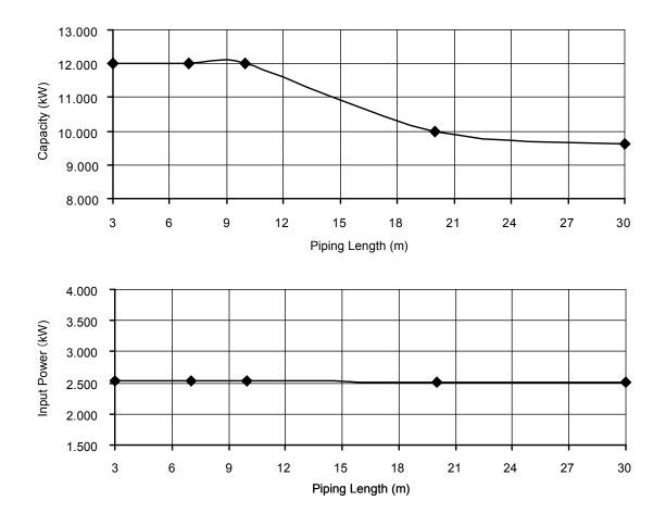
Cooling Characteristics at Different Piping Length Condition Outdoor air temperature : 35°C (DBT), -°C (WBT) Indoor water inlet temperature : 12°C Indoor water outlet temperature : 7°C Piping length : 7 m
