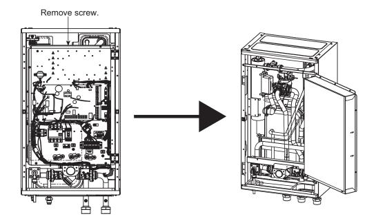
17.8 To Remove Pressure Relief Valve, Air Purge Valve and Flow Sensor
