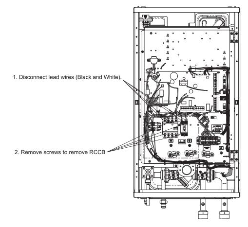
17.6 To Remove Transformer and Electronic Controller Board
