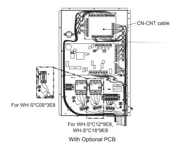
2. Insert a flat head screwdriver into the slot on the top of the adaptor and remove the cover. Connect the other end of the CN-CNT cable connector to the connector inside the adaptor.
