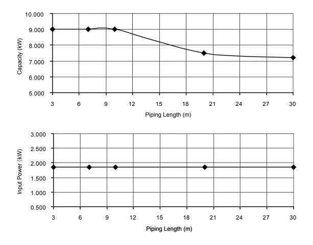
**Cooling Characteristics at Different Piping Length**
