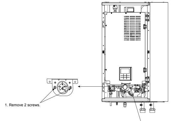
2. Use spanner to release nut of pressure gauge
