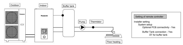
This is an application that connects the buffer tank to the indoor unit. Buffer tank's temperature is detected by buffer tank thermistor (specified by Panasonic). This system requires optional PCB (CZ-NS4P).
