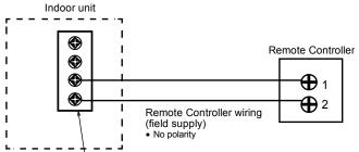
Terminal for Remote Controller wiring
