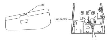
3. On the wall near the Indoor Unit, attach the adaptor by screwing screws through the holes in the back cover.
