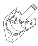
Use test pen to push this button for reset Overload protector (11).
