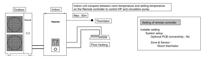
Connect floor heating or radiator directly to indoor unit.
