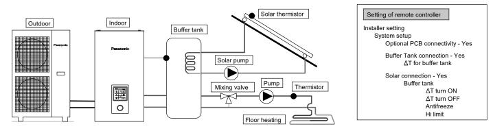
This is an application that connects the buffer tank to the indoor unit before connecting to the solar water heater to heat up the tank.
