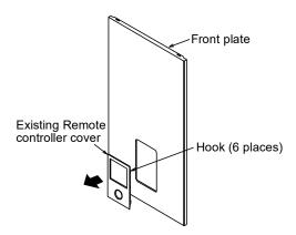
Press from front to fix the Remote controller cover
