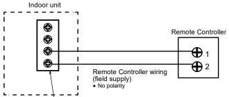
Terminal for Remote Controller wiring
