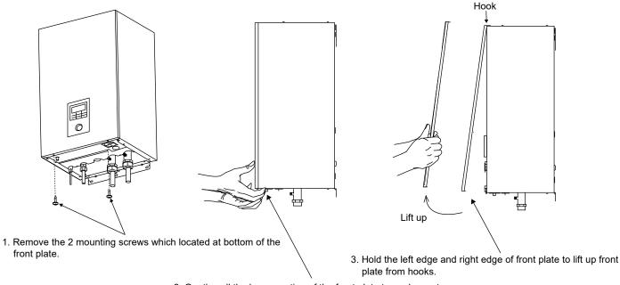
2. Gently pull the lower section of the front plate towards you to remove the front plate from left and right hooks.
