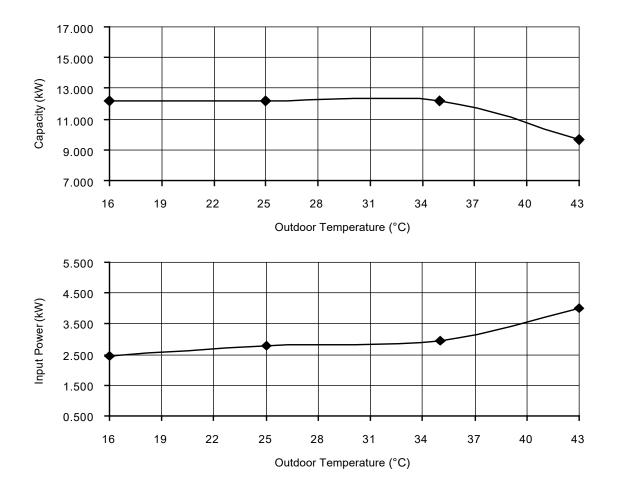
Heating Characteristics at Different Piping Length
