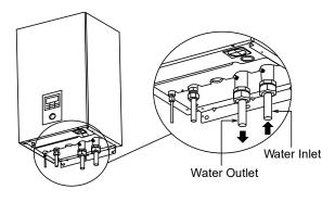
Do not over tighten, over tightening cause water leakage.
