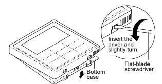
2. Remove the wiring between Remote controller and Indoor Unit terminal. Remove the bottom case from the Control board cover by loosening the screws. (3 pieces)
