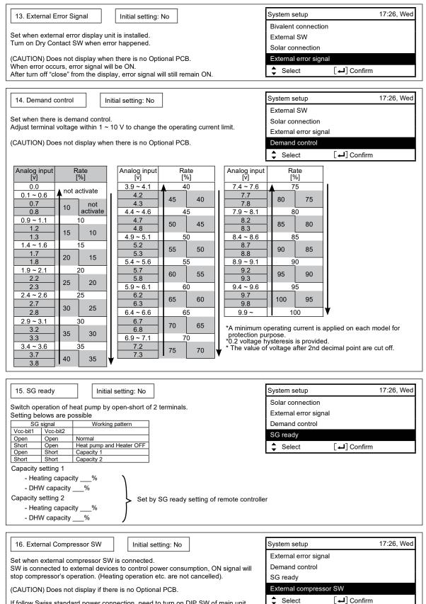
If follow Swiss standard power connection, need to turn on DIP SW of main unit PCB. ON/OFF signal used to ON/OFF tank heater (for sterilization purpose)
