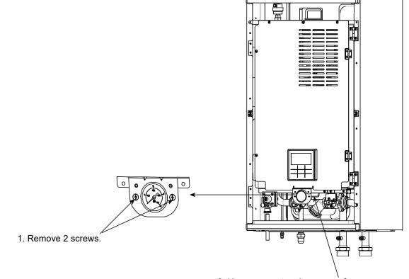
2. Use spanner to release nut of pressure gauge
