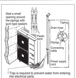
Seal a small opening around the pipings with gum type sealant.
