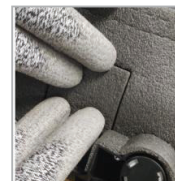
⑧ Put Insulator
