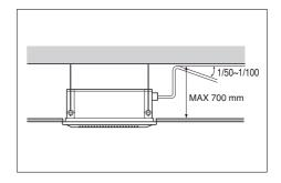
3. 5 mm or thicker formed thermal insulator is provided for the drain pipe.
