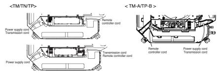
· While connecting wired remote controller, insert#ts connector to the "CN-REMO" housing of the main PCBA and make the remote controller cord tightly by using clamp cord.
