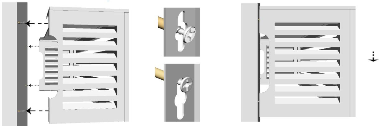
If you want to take off the cover, please increase the height slightly according to the position of the screw holes, and simply pull it outward through the middle of the last hole position of the drawing. This is a simple installation that also allows for quick removal of our cover for system maintenance.
