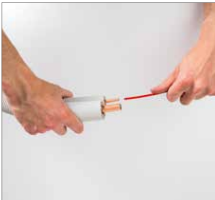
Step 1: Insert the flexible bender of the right diameter into the copper tube
