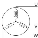
Measure the resistance between the terminals with a multimeter (at the ambient temperature 20°C).
