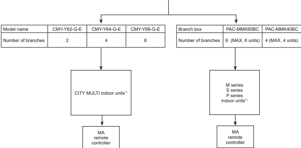
\*1. Refer to "System construction" or "System construction (Branch box system)", for more detail.
