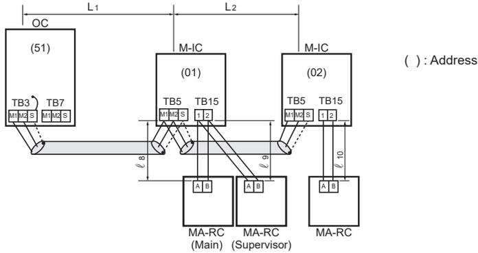
Using 2 MA remote controllers with alarm for CITY MULTI series indoor unit.
