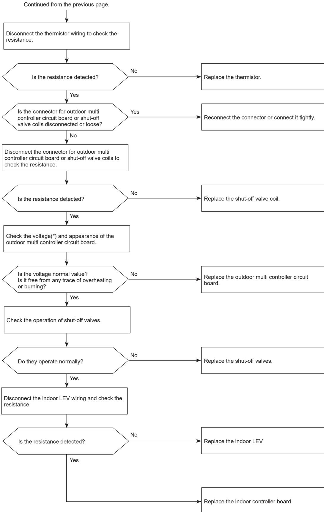
\*For the voltage, refer to "How to check the components".
