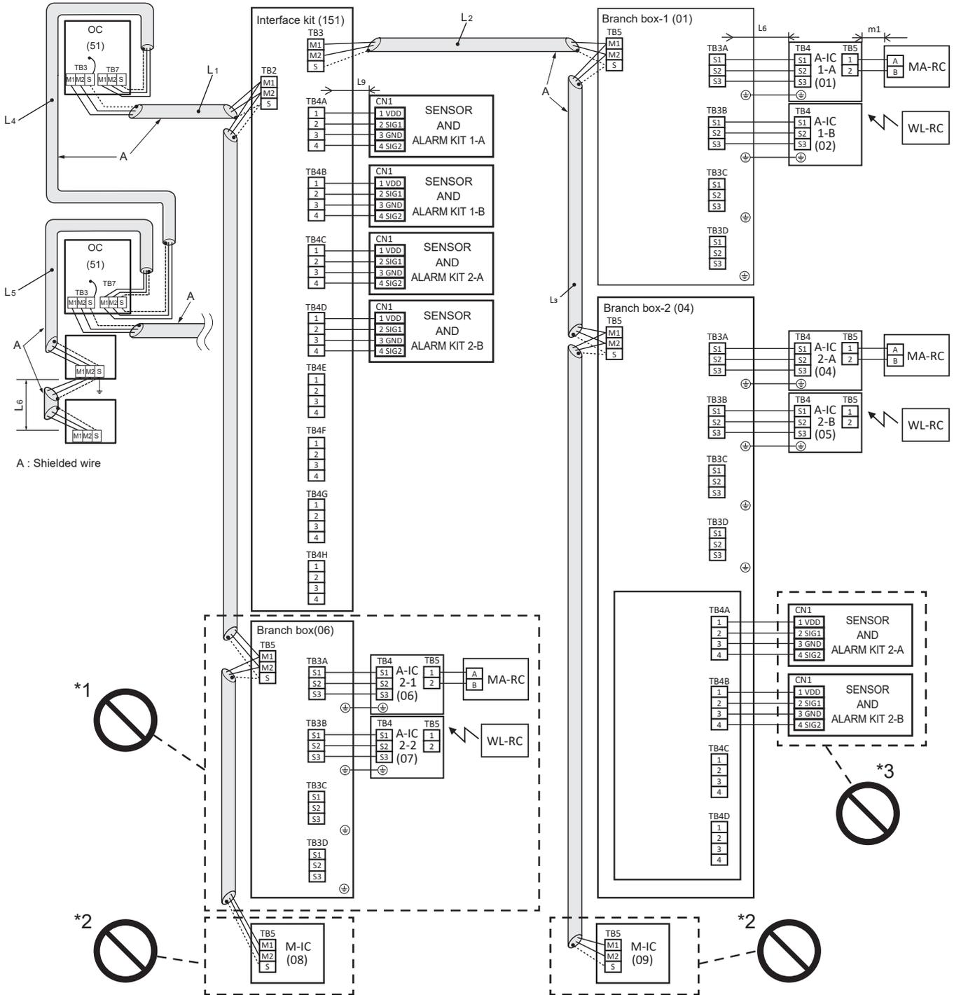
\*1. When connecting interface kit, it is not possible to connect a Branch box without through the interface kit.
