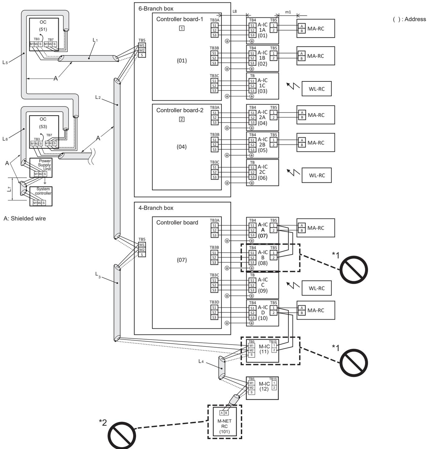
Different refrigerant systems cannot be connected together.
