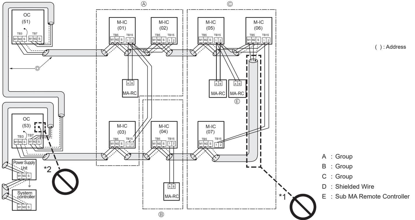
M-NET remote controller and MA remote controller cannot be connected with the CITY MULTI series indoor unit of the same group wiring together.
