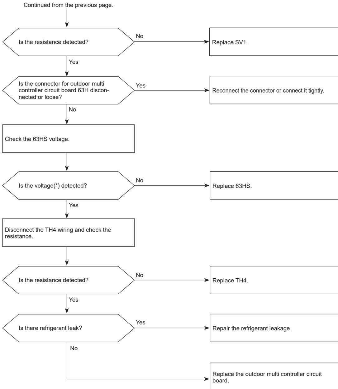
\*For the voltage, refer to "How to check the components".
