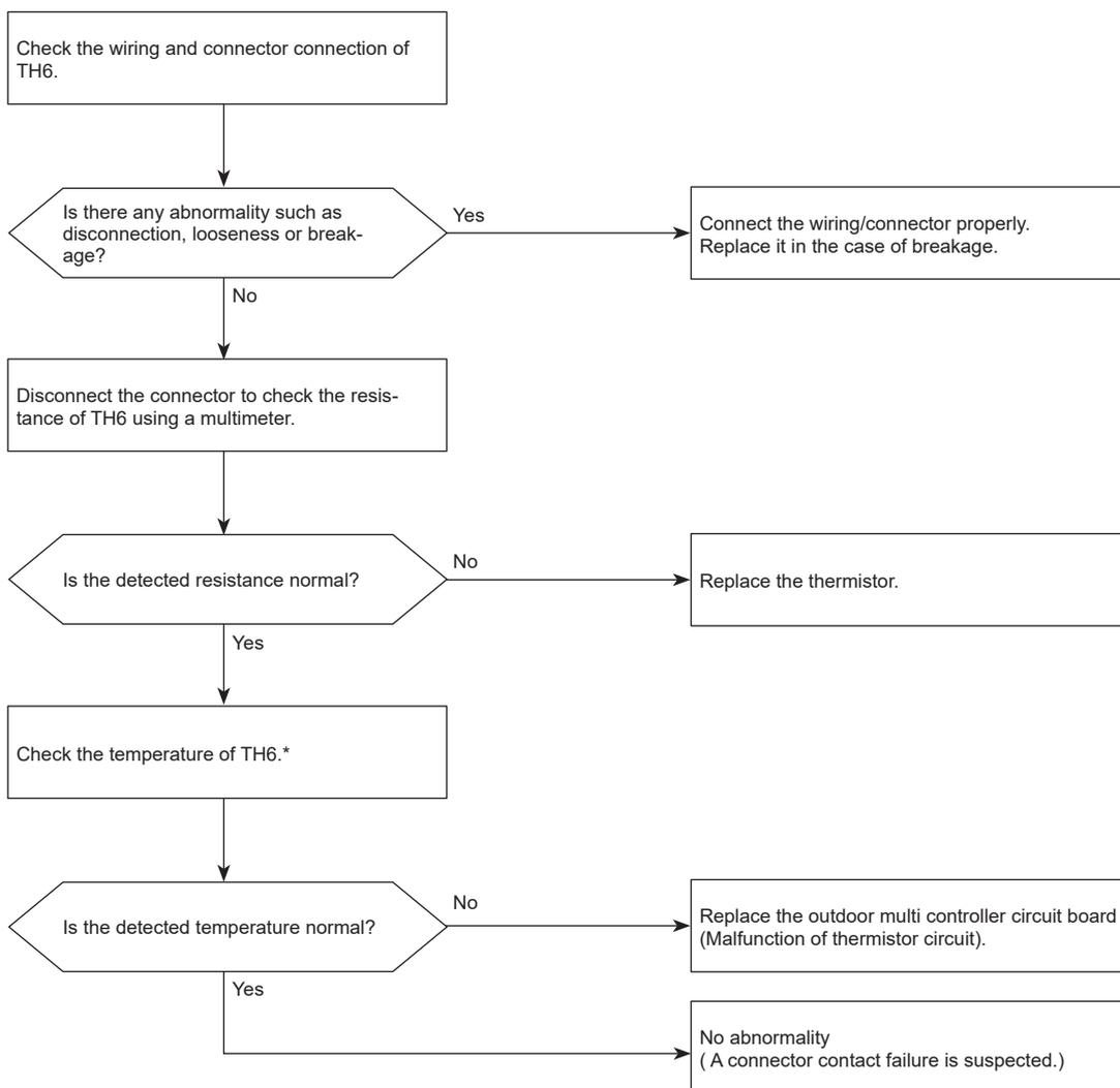
\* The detected temperature of TH6 can be displayed by an operation of SW4 on the outdoor multi controller circuit board.
