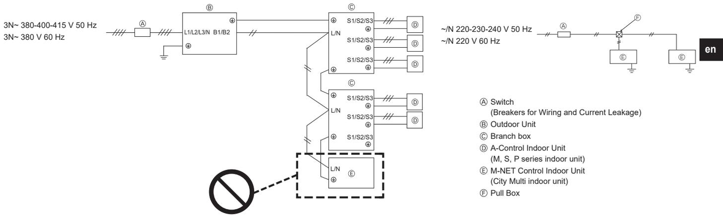
\* The M-NET Control Indoor unit cannot receive power supplied from an outdoor unit, so provide it with power separately.
