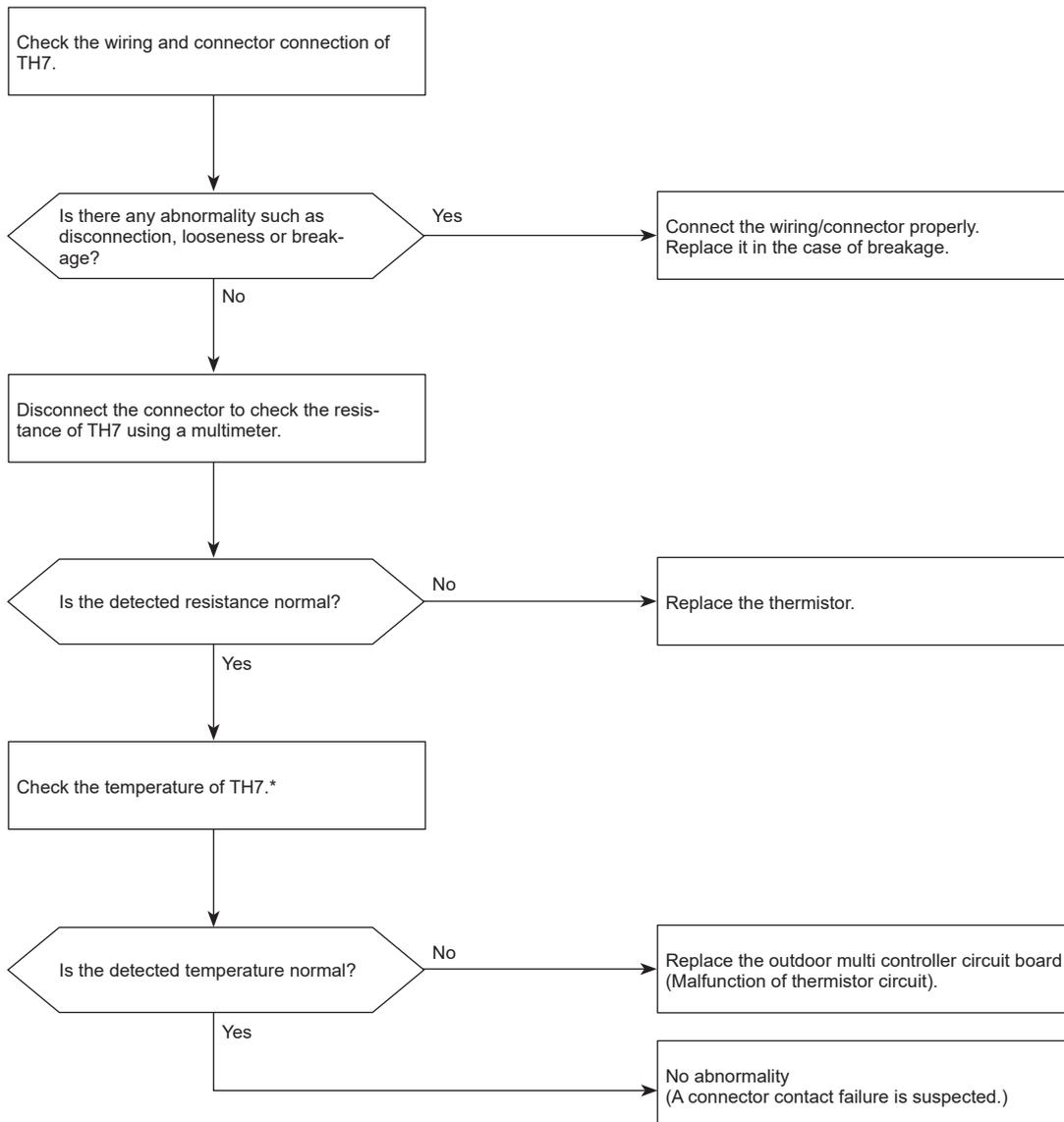
\* The detected temperature of TH7 can be displayed by an operation of SW4 on the outdoor multi controller circuit board.
