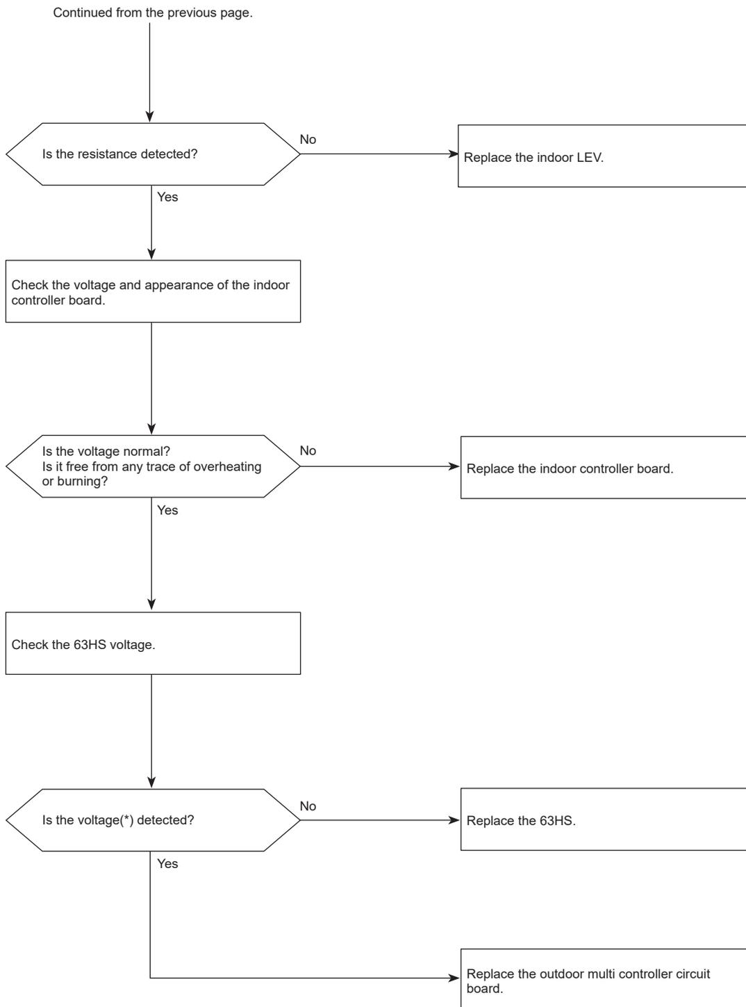
\*For the voltage, refer to "How to check the components".
