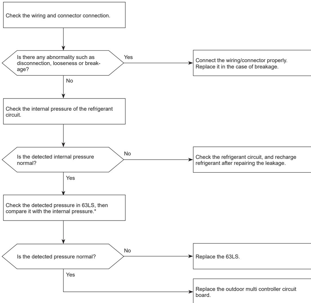
\* The detected pressure in 63LS can be displayed by an operation of SW4 on the outdoor multi controller circuit board.
