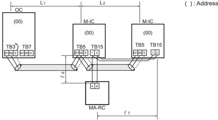
Multiple indoor units operated together by 1 MA remote controller.
