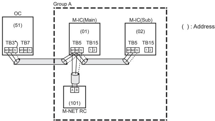
Multiple CITY MULTI series indoor units operated together by 1 M-NET remote controller.
