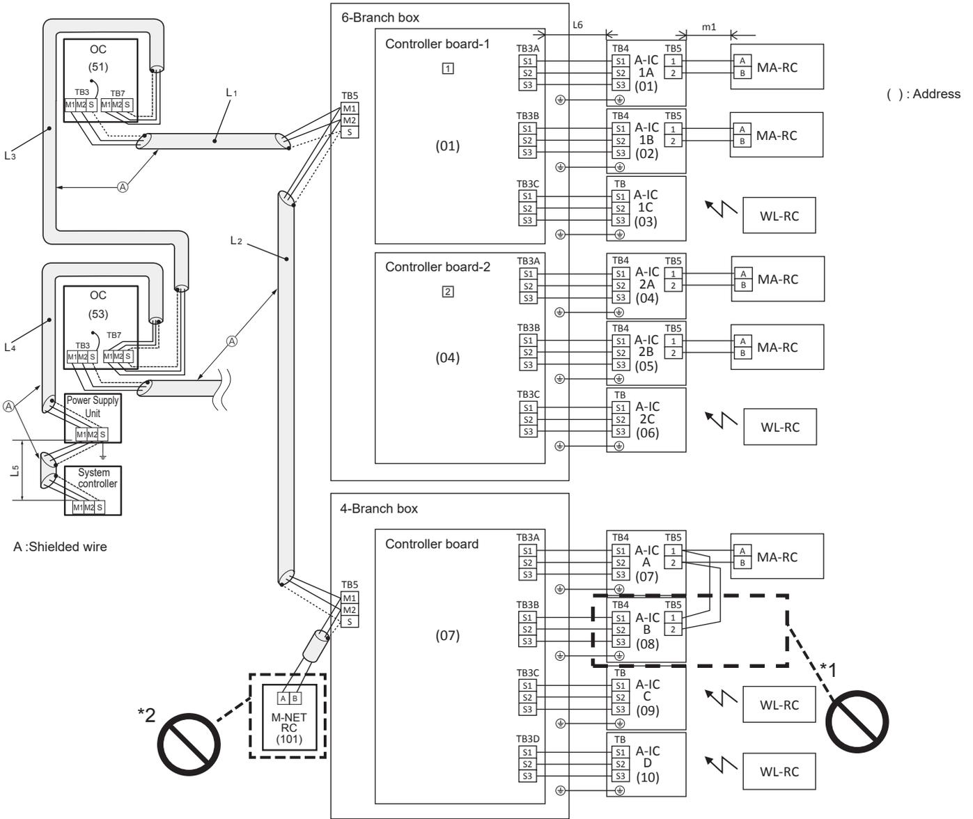
Different refrigerant systems cannot be connected together.
