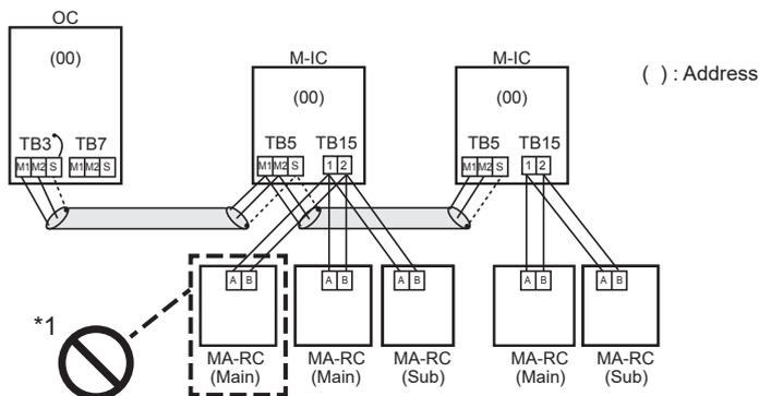
\*1. 3 MA remote controllers or more cannot be connected with the CITY MULTI series indoor unit of the same group.
