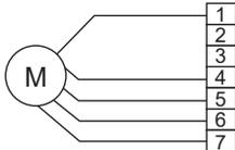
Measure the resistance between the connector pins with a multimeter (at the ambient temperature 20°C).
