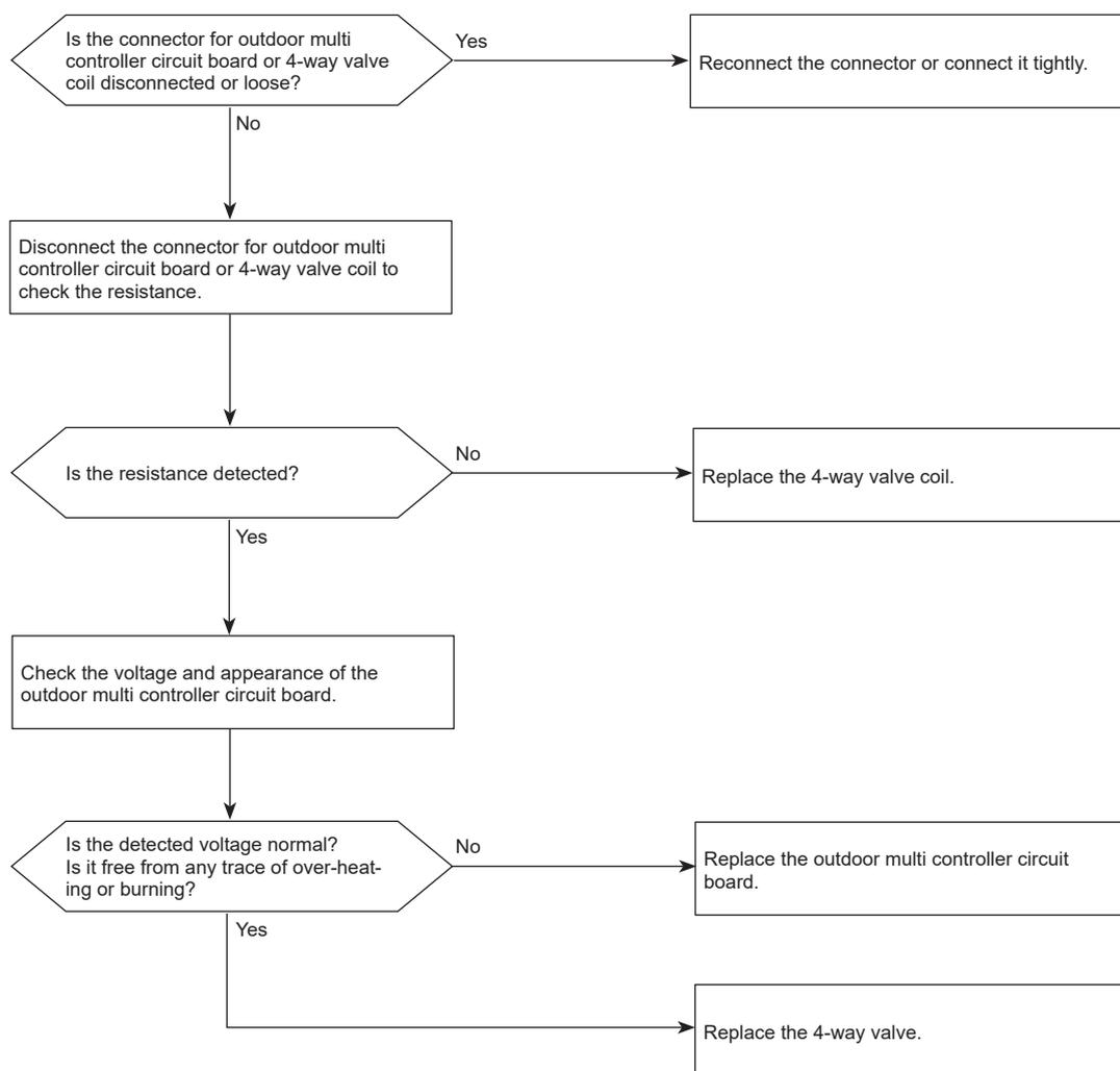
Refer to "How to check the parts" for ohm values.
