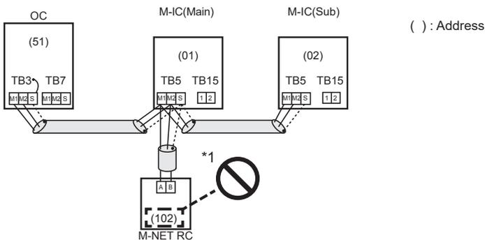
\*1. The M-NET remote controller address is the CITY MULTI series indoor unit main address plus 100. In this case, it should be 101.
