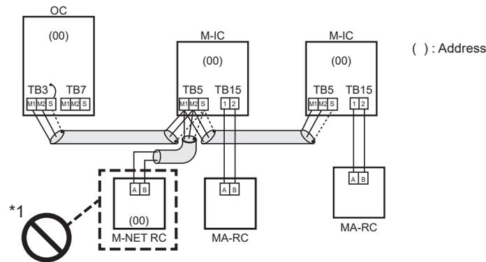
\*1. The MA remote controller and the M-NET remote controller cannot be used together with the CITY MULTI series indoor unit of the same group.
