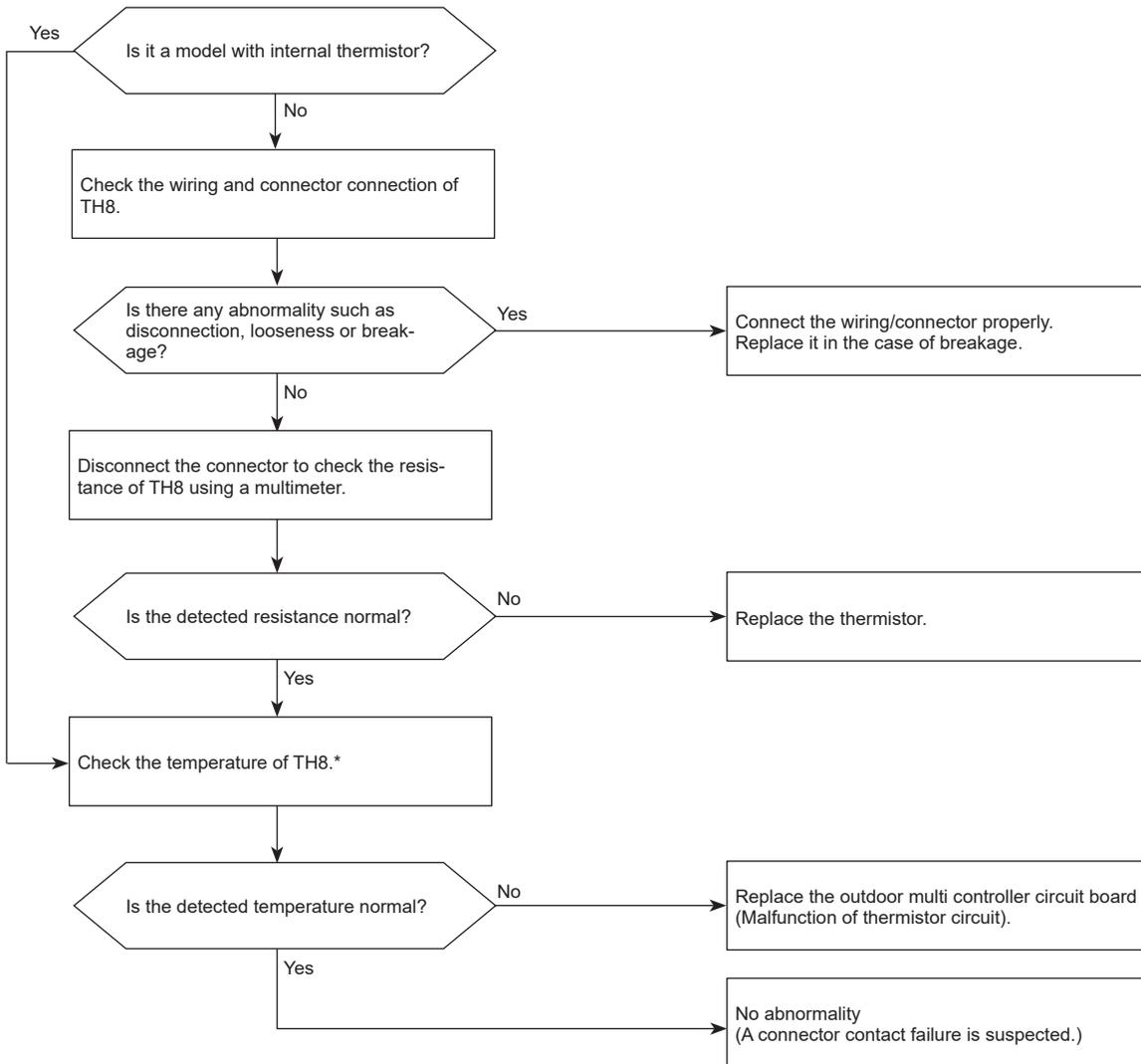
\* The detected temperature of TH8 can be displayed by an operation of SW4 on the outdoor multi controller circuit board.
