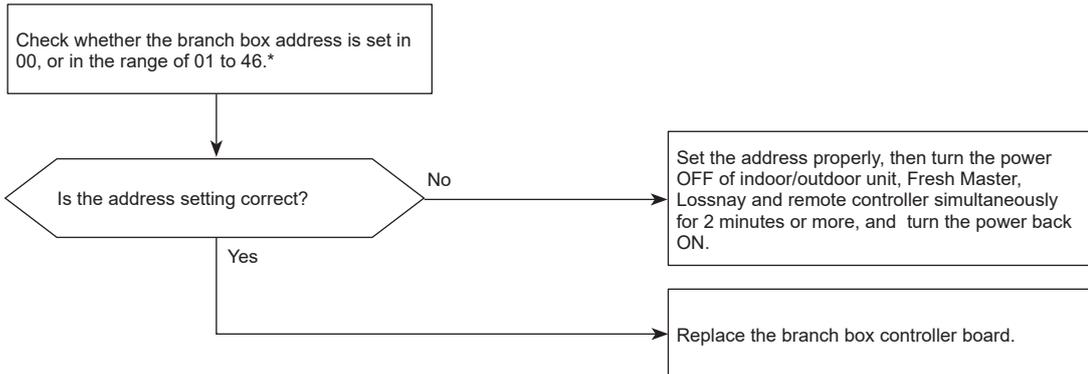
\* Branch box port addresses are set sequentially and they must not exceed 50. For example, when 5 indoor units are connected and the branch box address (port A address) is set to 47, it is not allowable because the port E address exceeds 50 (A: 47, B: 48, C: 49, D: 50, E: 51).
