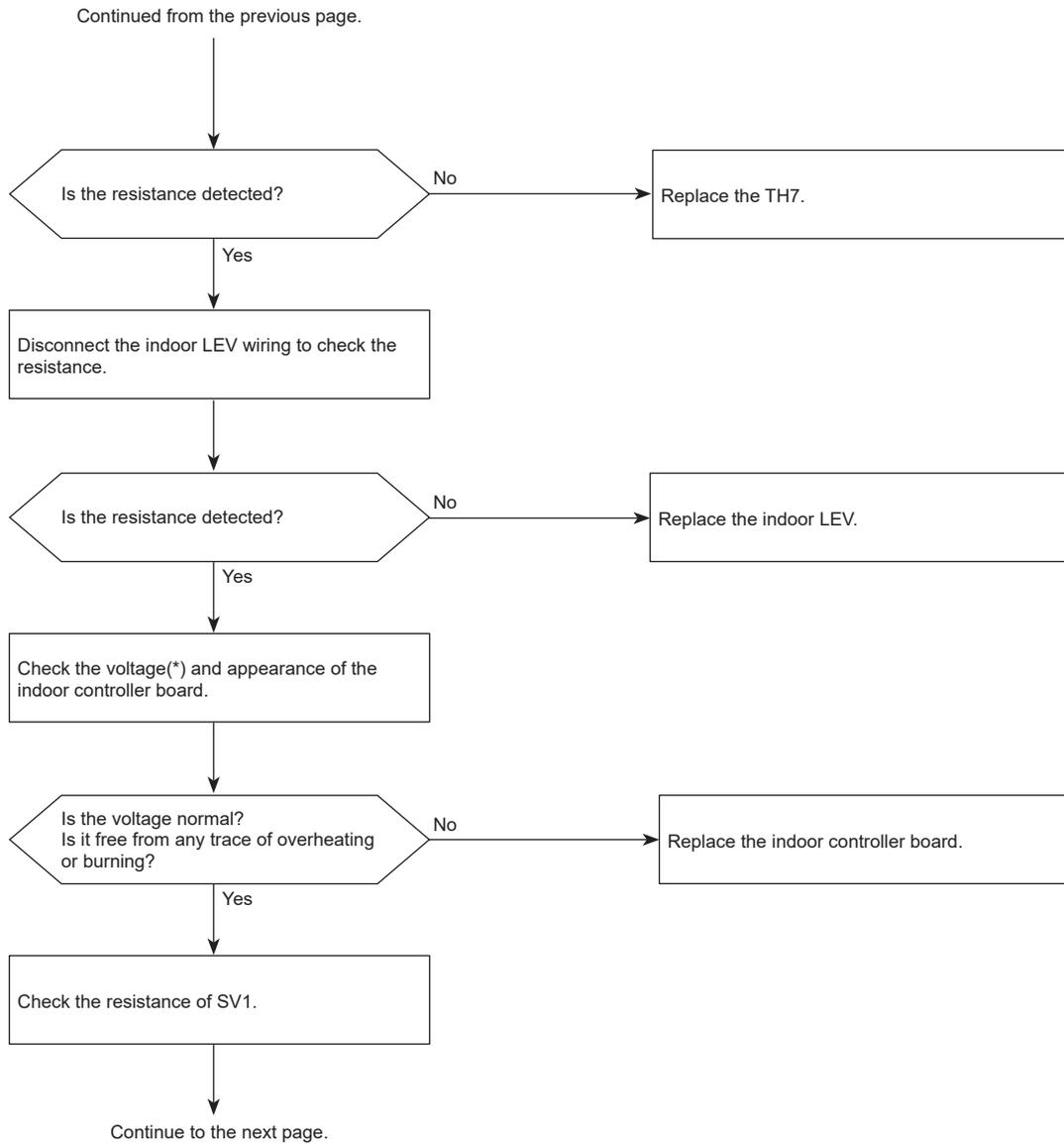
\*For the voltage, refer to "How to check the components".
