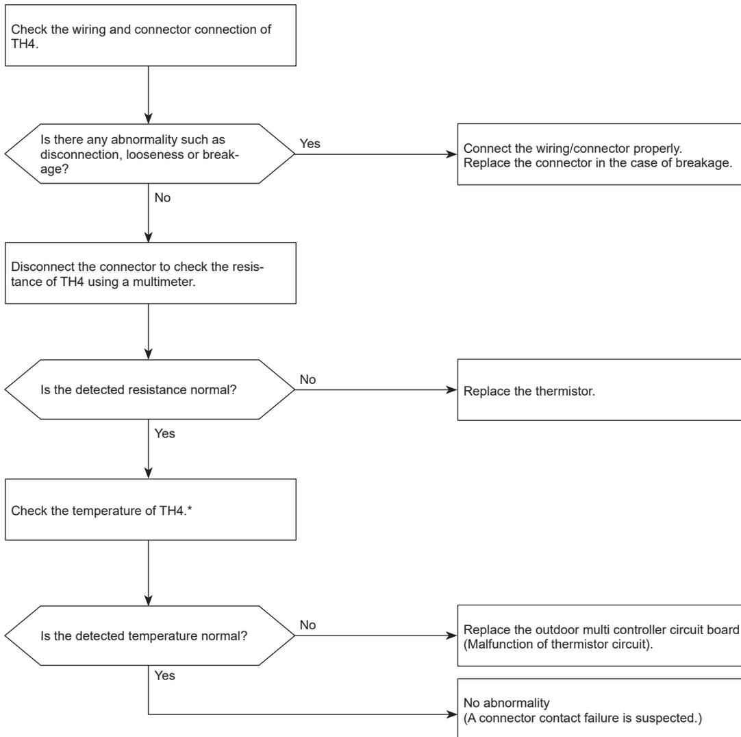
\* The detected temperature of TH4 can be displayed by an operation of SW4 on the outdoor multi controller circuit board.
