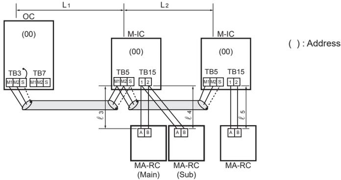
Using 2 MA remote controllers for each CITY MULTI series indoor unit.
