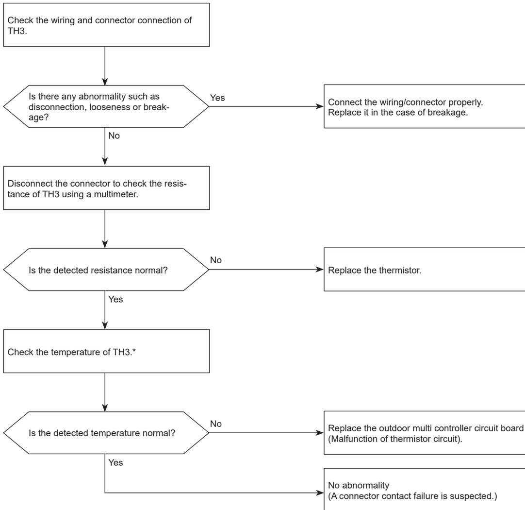
\* The detected temperature of TH3 can be displayed by an operation of SW4 on the outdoor multi controller circuit board.
