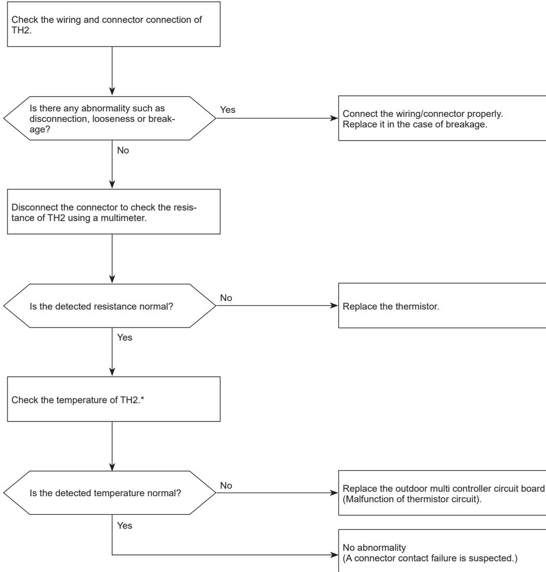
\* The detected temperature of TH2 can be displayed by an operation of SW4 on the outdoor multi controller circuit board.
