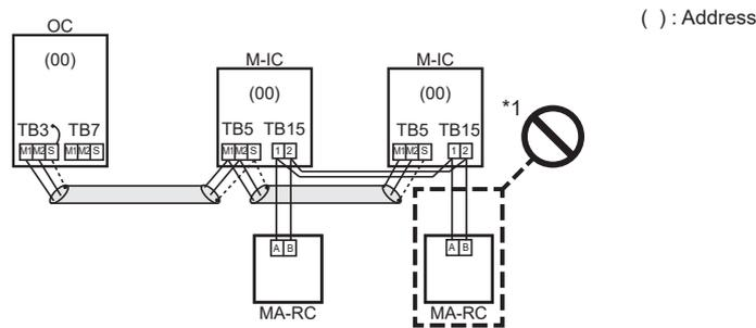
\*1. The second MA remote controller is connected with the terminal block (TB15) for the MA remote controller of the same CITY MULTI series indoor unit (M-IC) as the first MA remote control.
