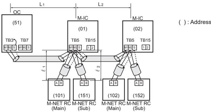
Using 2 M-NET remote controllers for each CITY MULTI series indoor unit.
