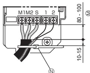
Secure the remote controller cable and indoor-outdoor connection cable with the cable strap.
