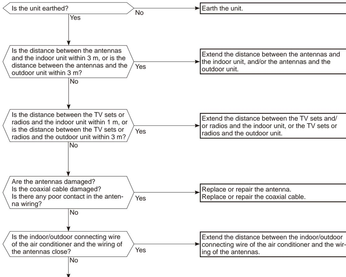
Even if all of the above conditions are fulfilled, the electromagnetic noise may enter, depending on the electric field strength or the installation condition (combination of specific conditions such as antennas or wiring). Check the following before asking for service.
