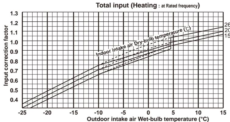
**NOTE:** The above broken lines are for the heating operation without any frost and defrost operation.
