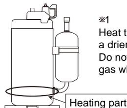
※1 Heat the compressor with a drier for about 20 minutes. Do not recover refrigerant gas while heating.
