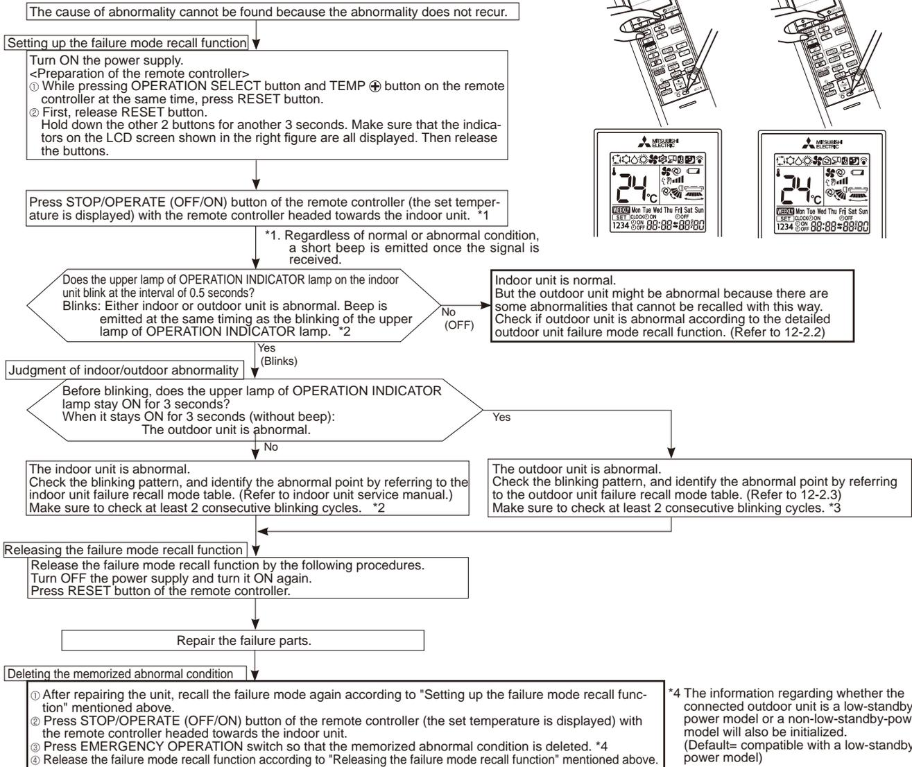
**NOTE:**1. Make sure to release the failure mode recall function after it is set up, otherwise the unit cannot operate properly.
