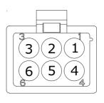
riangle Note that the position is mirror faced in comparison to the electrical connections. For example, position 1 on the cable is referring to PIN 3 on the electrical connector on the sensor.
