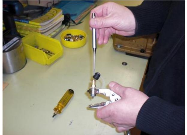
Punch out the old piercing needle tip with an appropriately sized punch from the back by going through the center of the brass fitting using a punch and a hammer.
