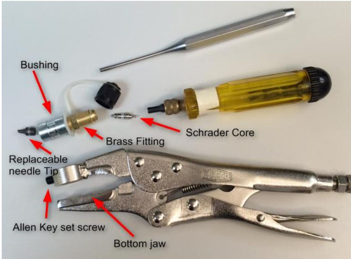
Remove the Schrader core from inside the brass fitting using a Schrader core removal tool (For example the REFCO A-32000).
