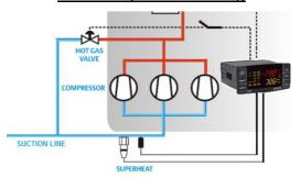
To detect the suction superheat an auxiliary probe among P3 (term. 3-4) or P4 (term. 33-34) has to be set as superheat temperature probe.
