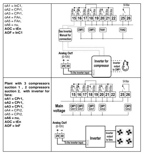
CtyP Compressor type: it sets if compressors have the same power (homogeneous) or not.
