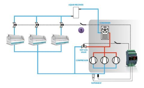
To enable this function set one relay by the parameters oA2 or oA3 or oA4, as flood protection, El **oA4 = Lig.** and then connect it to the external device that blocks the cabinet injection. NOTE: the relay set as flood protection is automatically activated even when the controller is in
