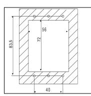
Keyboard **VC660** shall be mounted on vertical panel, in a 72x56 mm hole, and fixed using screws  $\varnothing$  3 x 2mm. To obtain an IP65 protection grade use the front panel rubber gasket (mod. RGW-V).
