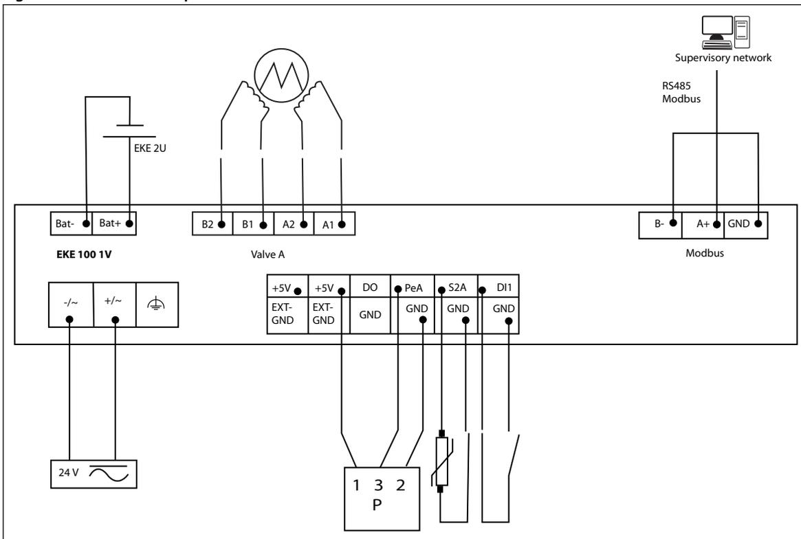
Figure 4: See below example for EKE 100 2V
