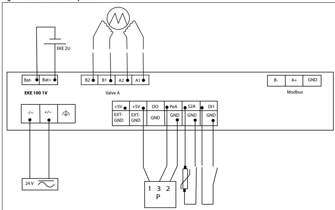
Figure 2: See below example for EKE 100 2V
