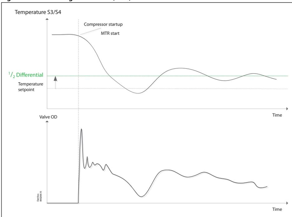
Offsetting Superheat, Opening degree and temperature via External signal
