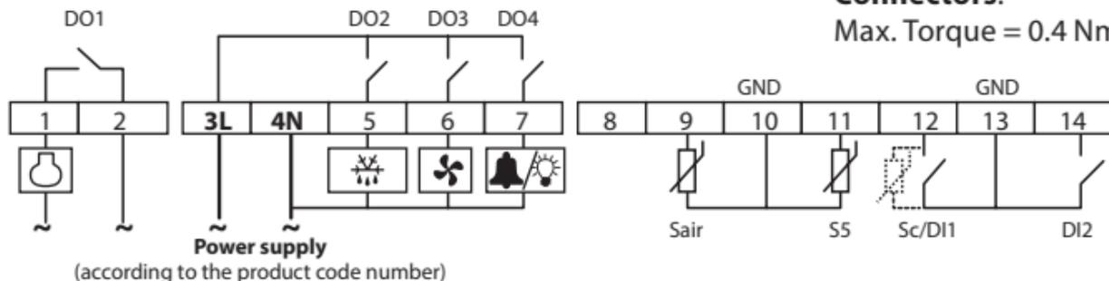
The **ERC 214** is a smart, multipurpose integrated refrigeration controller with temperature and defrost management, available with 4 relays.
