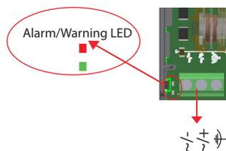
The image shows the position of the alarm/Warning LED.
