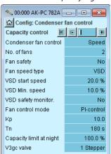
In our example we use a number of fans that are all speed-controlled in parallel. The settings are shown here in the display.
