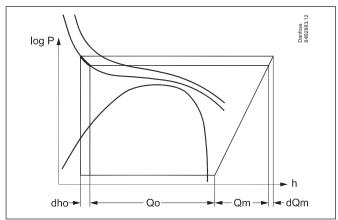
The function also increases the load on the compressor motor as pressure increases. Power consumption increases to Qm+dQm.
