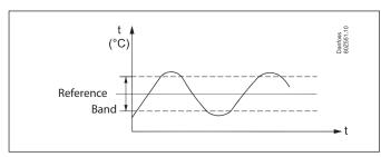
When the temperature goes above the reference plus the half band, the gas is routed around the heat exchanger.
