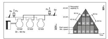
As the variable part of the speed controlled compressor is bigger than the following compressor steps, the capacity curve will be without holes.
