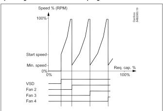
The controller starts the frequency converter and increases the speed of the first fan.
