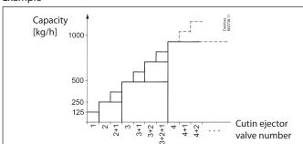
Shown here is the start of a "High pressure lift" control with four ejector valves. The total capacity can be controlled up to approx. 1875 kg/h.
