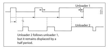
CRII 6: The pulse signal can also be used to control one CRII with three unloaders (6-cylinder version).
