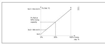
The minimum temperature difference (min tm) at low load should be set at approximately 2 K as this will eliminate the risk that all fans will be running when no compressors are running. Set the dimensioned difference (dim tm) at max. load (e.g. 4 K).
