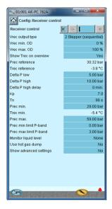
When the MT suction control is configured to alternate between two pressure transducers (P0-MT and Psuc-MT - typically used with Low Pressure Multi Ejectors), some of the receiver control parameters are unavailable and replaced by others. The reference for the receiver uses a higher or a lower offset, determined by a digital input. The new parameters are explained to the right. The remaining parameters are as explained on the previous page.
