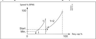
At low loads, only group 1 will be cut in. When the load increases and a calculated start value for group 2 is exceeded, group 2 will be started.
