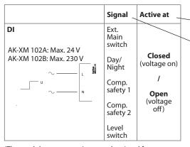
(The module can not register a pulse signal from e.g. a reset function.)
