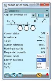
4. Set capacity in percentage Press in the blue field Manual capacity.
