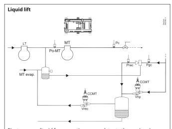
Ejectors move liquid from a suction accumulator to the receiver. In systems with LE and HP ejectors - depending on the ejector envelopes - either LE or HP ejectors will have priority to lift liquid. When liquid is not present, vapor will be lifted.
