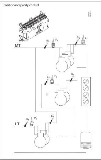
Heat recovery functions, controlling the condensing pressure and receiver pressure
