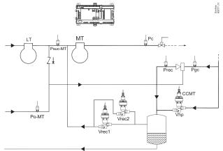
LP ejector control has no parallel compression.
