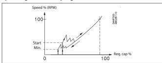
The controller starts the frequency converter and the first fan when the capacity requirement corresponds to the set starting speed.
