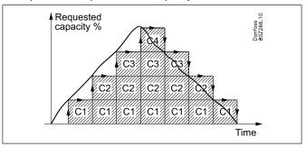
Cut-out of the last compressor stage:
