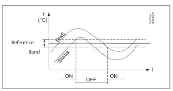
The pump is controlled via on/off and is connected when Stw8 is below the reference plus half the difference. It is disconnected when Stw8a is above the reference plus half the difference.
