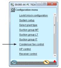
In our example, the condenser pressure is controlled on the basis of the Sgc and from Sc3 (floating reference).
