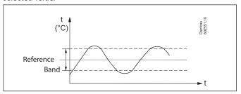
When the temperature goes above the reference plus half the band, the gas will be routed outside of the heat exchanger. The reference can be displaced variably using an external 0-10 V signal. 0 V result in no displacement. 10 V result in a displacement indicated by the set value.
