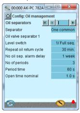
The process is as follows: When a signal is given from the level switch, the discharging process to the receiver commences. This pulsates three times with one minute intervals. Each pulse lasts one second. If the level switch does not register an oil drop at this point, an alarm is given when the delay time has expired.
