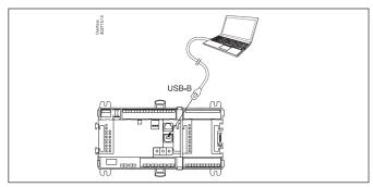
The controller must be switched on first and the LED "Status" must flash before the Service Tool program is started.
