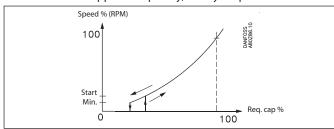
The controller starts the frequency converter when the capacity requirement corresponds to the set starting speed. The controller stops the frequency converter when the capacity requirement becomes lower than the set minimum speed.
