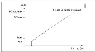
If the Sgc temperature exceeds the defined "Absolute Max Sgc temperature", the output voltage will be allowed to increase to the EC absolute maximum value.
