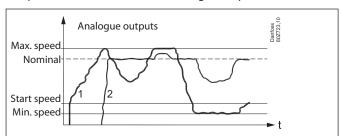
The first is run up to maximum speed. Number two is then activated and run up to nominal speed – and kept there. The speed of number one is reduced at the same time, so the capacity is balanced. All variations are now handled by number one. If number one reaches maximum speed, number two will also be raised.
