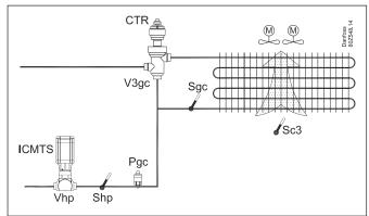
The pressure in the gas cooler is controlled by the Vhp valve. Instead of an ICMTS valve, an injector or a CCMT valve with stepper motor can be used.
