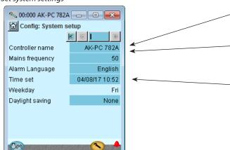
All settings can be changed by pressing in the blue field with the setting and then indicating the value of the required setting.
