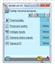
In our example we select one thermostat function for temperature control in the compressor room.
