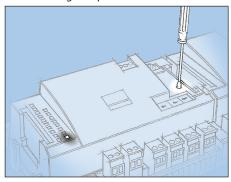
3. Wait for answer from the system unit Depending on the size of the network it may take up to one minute before the controller receives an answer as to whether it has been installed in the network. When it has been installed, the Status LED will start to flash faster than normal (once every half second). It will continue with this for about 10 minutes.
