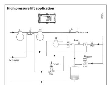
HP ejector control is an extension of the control with parallel compression. In this case, a part of the mass flow gets a high lift from MT suction group to IT compressors.
