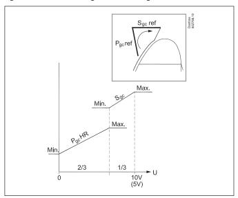
When heat recovery is activated (with a digital signal), the gas cooler pressure is increased to "Pgc HR min".
