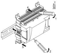
When the two snap catches for the DIN rail mounting are in the open position, the module can be pushed into place on the DIN rail – regardless of where the module is on the row. Disassembly is thus done with the two snap catches in the open position.
