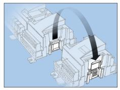
1. Remove the protective cap from the connection plug on the right-hand side of the basic module.
