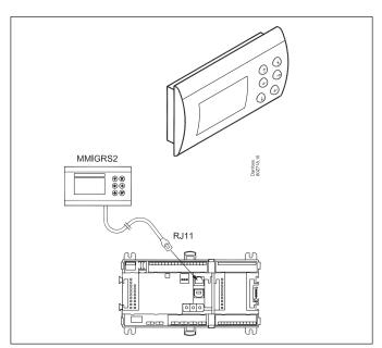
To create access, the display must be connected and the address of MMIGRS2 must be activated.
