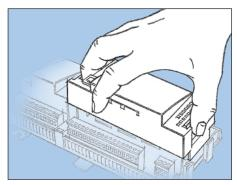
Press in the plate on the left-hand side of the light-emitting diodes and the plate on the right-hand side for the red address changers.
