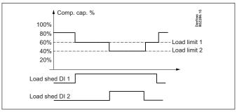
When both load-shedding signals are active, the lowest limit value for the capacity will be the one that is applicable.
